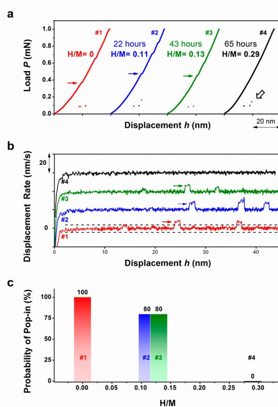
**Figure 2.** (a) Typical load displacement curves for indents in samples with different hydrogen content ( $c_H$ ). The curves are shifted for the sake of clarity. (b) Displacement rate as a function of displacement for each curve in (a). The first pop-ins are marked with arrows. The curves are shifted for the sake of clarity. (c) The percentage of indents that have no pop-in out of 144 tests in each sample.
