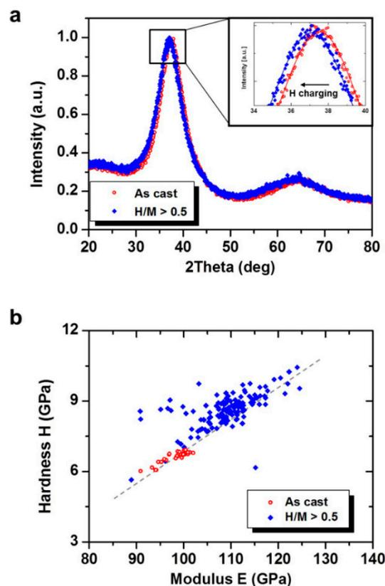
**Figure 1.** (a) X-ray diffraction spectra of Vit 105 metallic glass (MG) samples with and without hydrogen charging. The hydrogen content is defined as the hydrogen-to-metal ratio. (b) Hardness and modulus (Berkovich indentation) of samples with and without hydrogen charging. The dashed line is to guide the eye.
